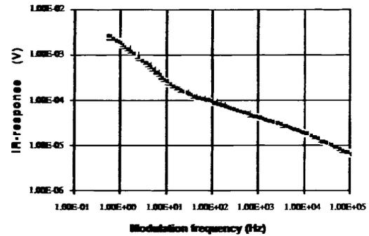
Fig. 6. IR-response versus modulation frequency of 0.05-cm thick SrTiO<sub>3</sub> substrate sample 064-01a measured at 0.25 mA bias currents. The measurement is done at 2.13 mW/cm<sup>2</sup> radiation intensity.
