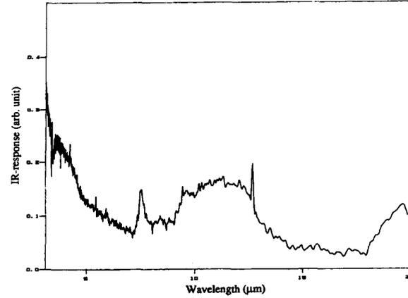
Fig. 3. Spectral response of sample 064-01a, up to 20- $\mu$ m wavelength (measured at EG&G, Judson Infrared Inc.). The response is measured at the middle of the superconducting transition with 0.55 mA bias current.
