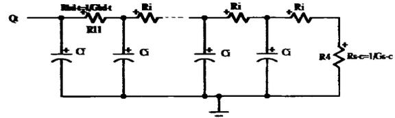
Fig. 4. Circuit diagram of thermal model for bolometric response of a high temperature superconducting bolometer.
