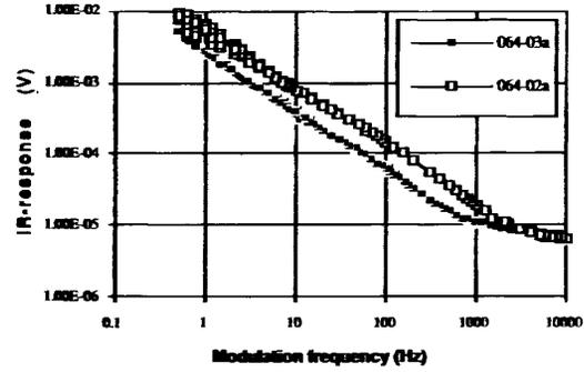
Fig. 5. Measured IR-response versus frequency for 0.05-cm thick MgO substrate sample 064-03a and 0.025-cm thick MgO substrate sample 064-02a. The measurements are done at middle of the superconducting transition with 1 mA dc bias current and 2.13 mW/cm<sup>2</sup> radiation intensity.
