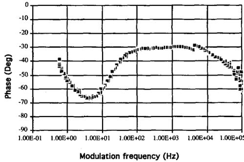
Fig. 7. Phase of IR-response versus modulation frequency of sample 064-01a (0.05-cm thick SrTiO<sub>3</sub> substrate) under the conditions given in Fig. 6.
