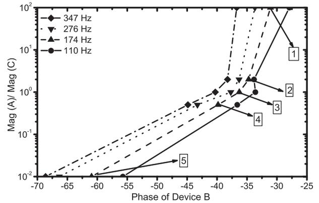
Fig. 3.  $\text{Mag(A)}/\text{Mag(C)}$  versus phase of readout device B. By measuring the phase of device B,  $\text{Mag(A)}/\text{Mag(C)}$  can be obtained. The numbers in squares show the calibration data points.
