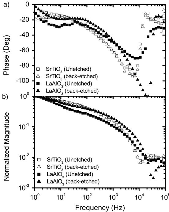
Fig. 5. (a) Phases and (b) magnitudes of back-etched and unetched bolometers made on  $LaAlO_3$  and  $SrTiO_3$  substrates.
