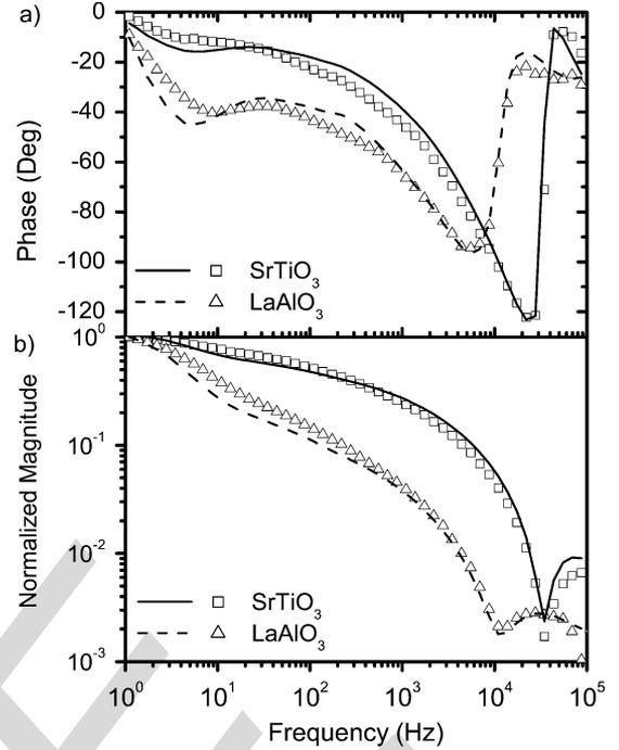
Fig. 4. (a) Phases and (b) magnitudes of pixels C on LaAlO<sub>3</sub> and SrTiO<sub>3</sub> substrates and their fitting curves.
