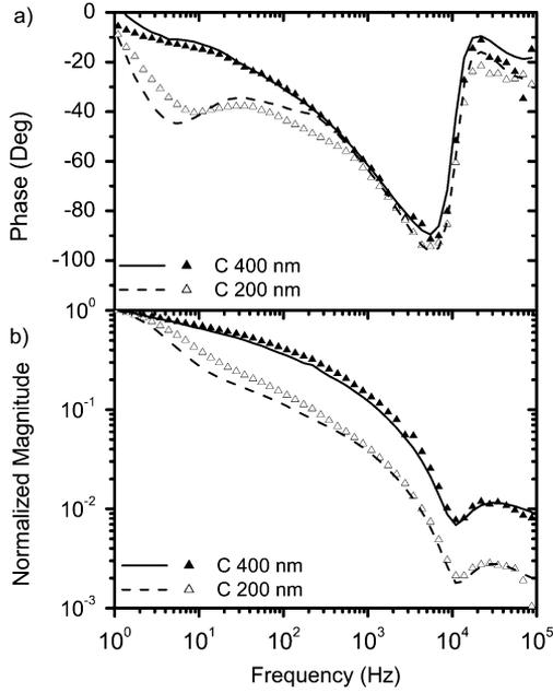
Fig. 3. (a) Phases and (b) magnitudes of 200- and 400-nm-thick bolometers and their fitting curves.
